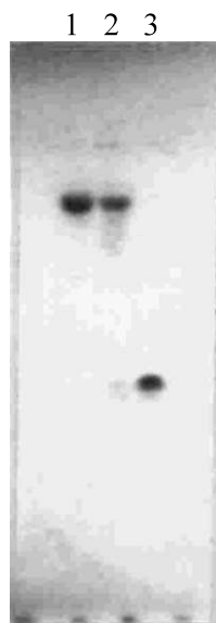
Figure 2. Photograph of 15% denaturing PAGE. Lane 1, O2-P1 ; lane 2, contaminated O2-P1 ; lane 3, O2 .
